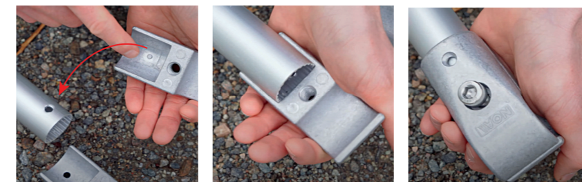
1. Position the spike to the hole on the tube 2. Hold the half with thread and spike 3. Put on the second half and fasten hex screw
